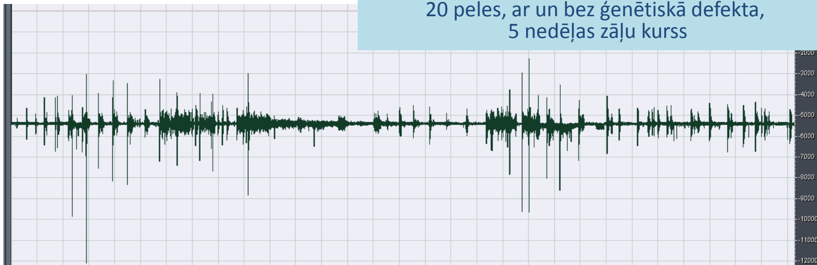
2023.04. Mouse vibration tremor sensing with home-built tensometric transducer force sensor scale.
