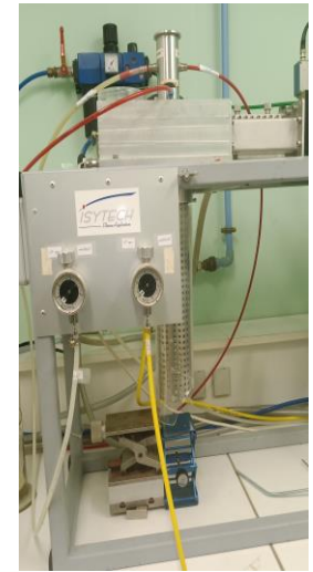
Setup for sphere fabrication from powders using plasma
