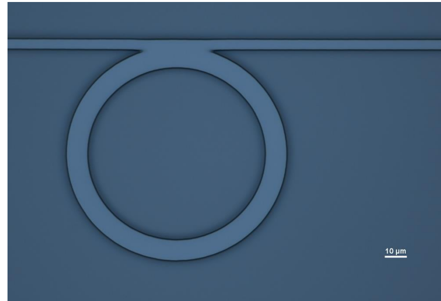
SU-8 polymer microring resonator photonic chip fabricated at the UL ISSP
